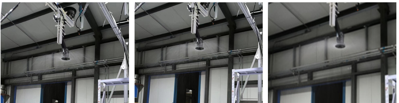
Figure 12 Test site of droplet size spectrum under the action of single rotor downwash flow field
