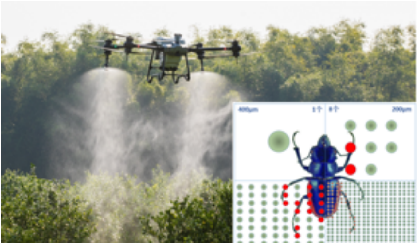
Figure 65 Fruit tree operations require higher dosage and finer droplets to ensure the effect
