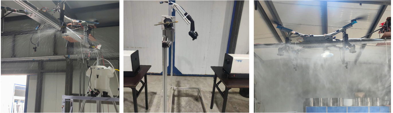
Figure 14 Test site of droplet size distribution in drone downwash flow field
